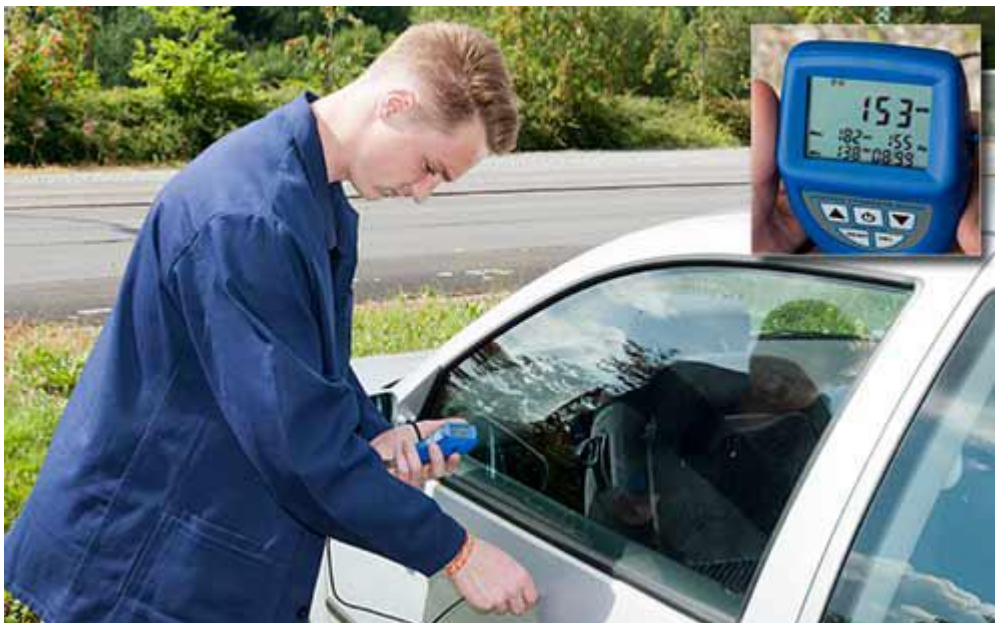
Here you can see the coating analyzer PCE-CT 27 during analysis of lacquer at a spot with a normal thickness of the coating
