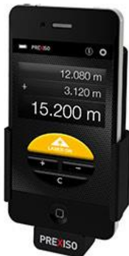
As soon as the iPhone laser telemeter iC4 is docked in the measurement can be initiated.
