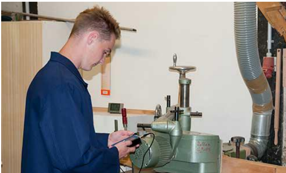
The vibration meter PCE-VM 3D during measurement on an engine
