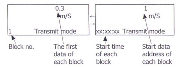
Use ▲ Up Button, ▼ Down Button to select the different data memory block no. ( 1 to 250 ).
