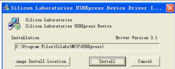
Click “Install” to finish the driver installation. After a successful installation of software and drivers, you can run the Vibration Datalogger software and communicate with the meter.
