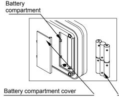
Remove the battery compartment cover and insert six batteries(R6P/LR6 /AAsize) into the battery compartment, taking extreme care that the polarities plus and minus is observed.
