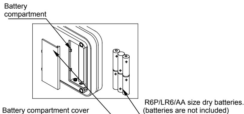
Remove the battery compartment cover and insert six batteries(R6P/LR6 /AAsize) into the battery compartment, taking extreme care that the polarities plus and minus is observed.
