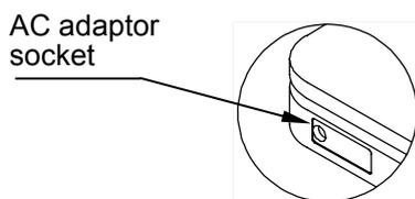
Plug the AC adapter to the AC adapter socket on the side. The AC input requirement could be 110,120,220,230 or 240Volts (50/60Hz) depending on the area where used, so please verify that the adaptor is correct
