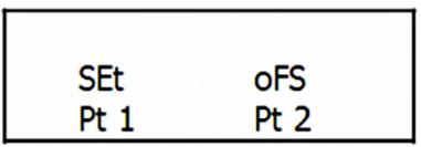
4) If you wish to make the offset adjustment for Pt 1, insert the probe into the PT1 input socket. Press the "L button" (4-5) once so that the display will show an example as follows. If you want to make the offset adjustment for Pt 2, insert the probe to the PT2 input socket. When you press the "R button" (4-6) once, the display will show an example as follows:
