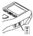
Insert the connector of the sensor into this socket. Either use the contact adaptor, an optical sensor or a magnetic sensor with an amplifier.
