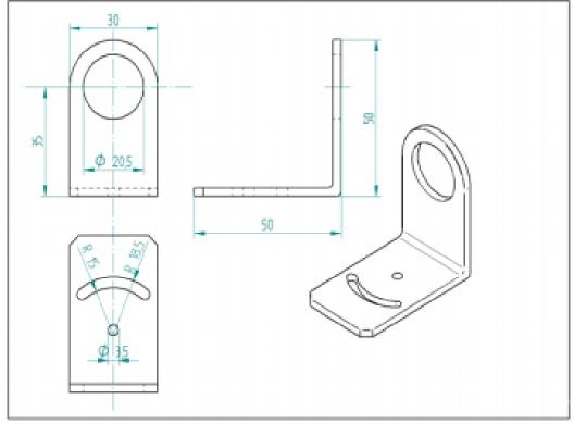
Dimensions of the three-dimensional installation equipment
