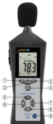
When you measure at wind velocities of  $>10\text{m/s}$ , use the wind protection on the microphone.
