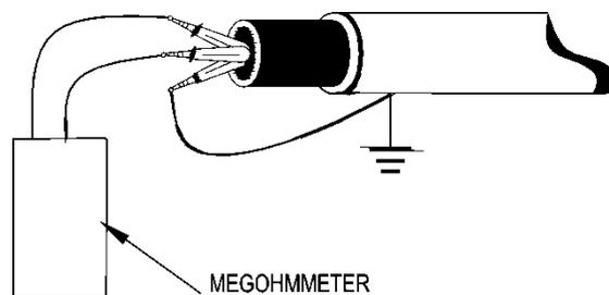
In this direction will find a vision of the measurement technique:
