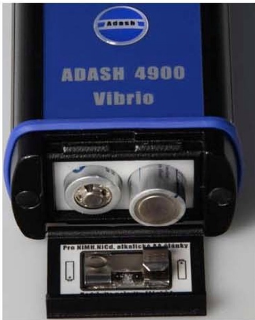
Fig. Placement of power batteries
