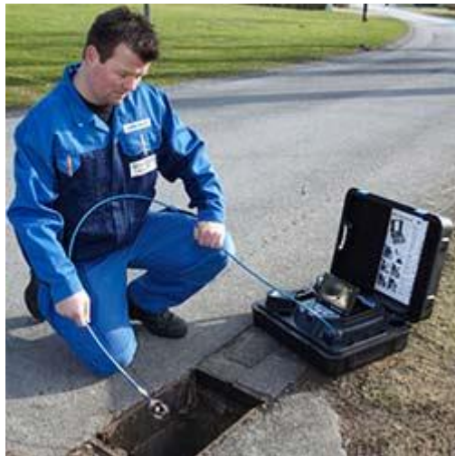
Here you can see the VIS 300 / 350 Endoscope inspecting a canal system.
