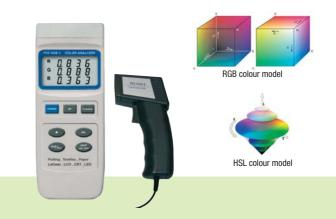
circular illumination 45°/ 0° by 45°, 0° measurement according to DIN5033
