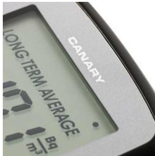
Display with indicator (dot at the upper right corner) of Radon-Monitor Canary.
