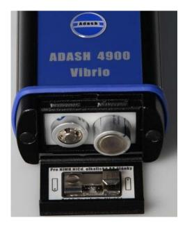
Fig. Placement of power batteries
