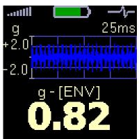
The time signal of bearing vibrations is displayed.  $g_{\text{ENV}}$  value is under the time signal (envelope modulated signal - see Methods for ball bearing condition diagnostics chapter. Caution – the time signal is displayed as a direct record, not after envelope modulation. Look at three basic screens for easy work with this function.
