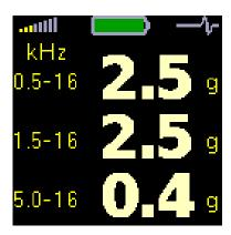
While in the last band the vibration value is very low, in the first two frequency bands the values are very high.
