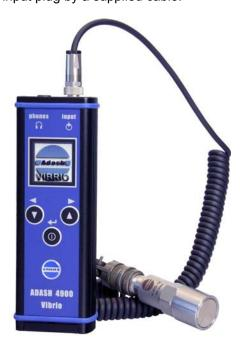
Fig. The instrument with a sensor connected
