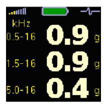
**The transmission is OK** and tooth frequency of 1,6 kHz slightly increases vibrations in the first two frequency ranges.
