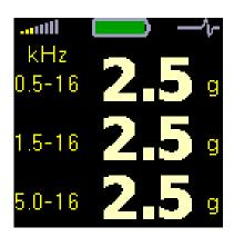
Vibrations are concentrated in the last frequency range 5 - 16 kHz, the vibrations in the last area are the same as in the area, where the tooth frequency shows itself - **bearing failure**
