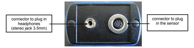
Fig. Top view of connectors
