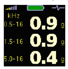
When we need to find the failure on not simple machines (e.g. gearbox) then is very usefull to know the vibration values in several frequency bands.
