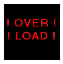
If an input signal is too strong (higher than 12V peak), and the instrument cannot process it, the overload error is displayed. The instrument is not capable of measuring this signal.
