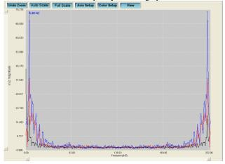
The software computes real-time spectral data using an FFT from 0 to 256 HZ.
