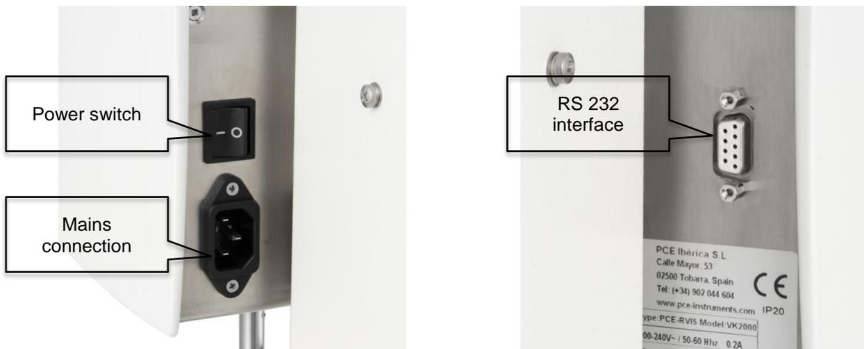
Power switch, mains connection and RS 232 interface are located at the back of the viscometer.
