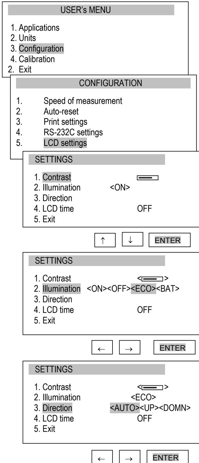
Use the navigation keys and *ENTER* to select *LCD settings*. Next, use *→*, *←* and *ENTER* to set the contrast at which the display is best legible.
