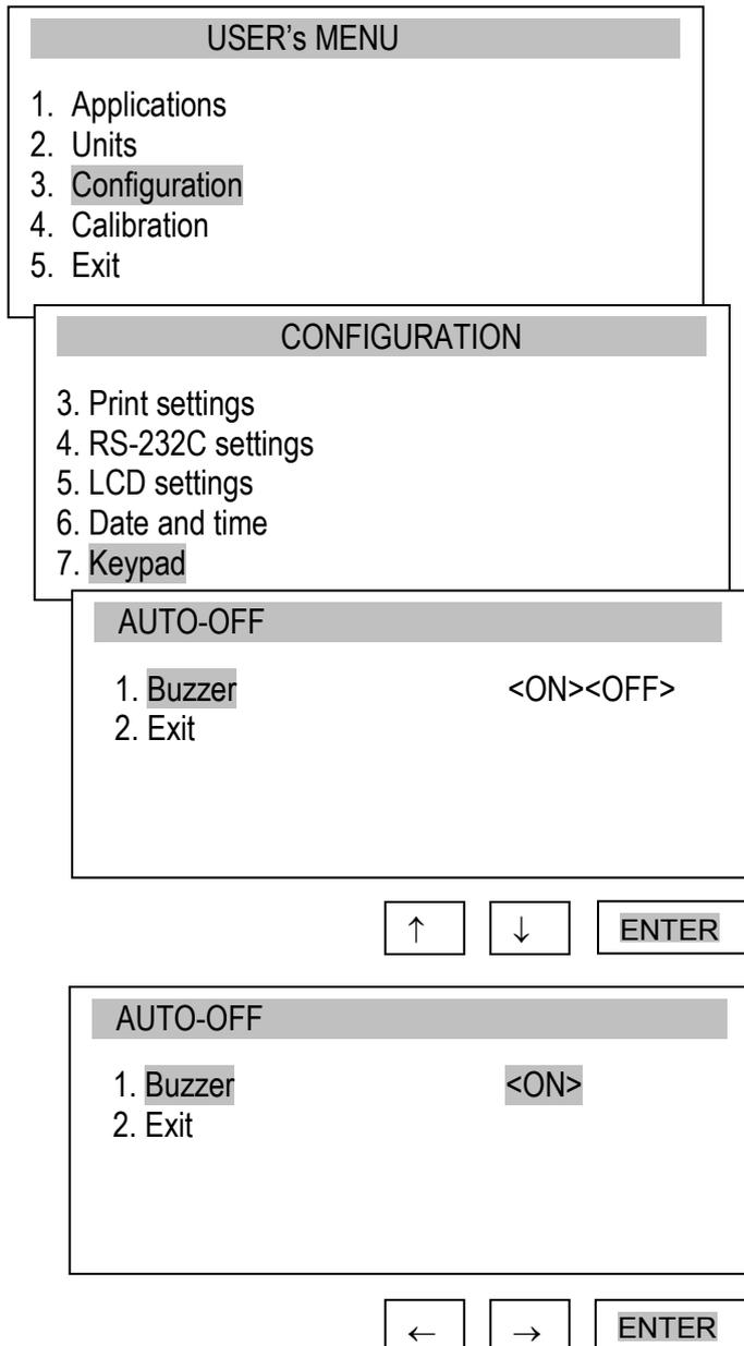
Use the navigation keys and *ENTER* to select *Keypad* and *Buzzer*, and one of the following options:
