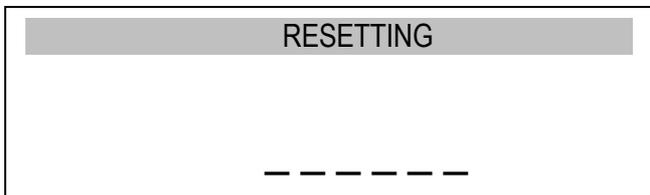
Reset the gauge in the operating position by pressing the  $\rightarrow T(0) \leftarrow$  key.
