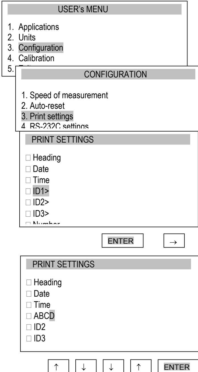
Use the navigation keys and *ENTER* to select *Print settings* and the suitable print components.
