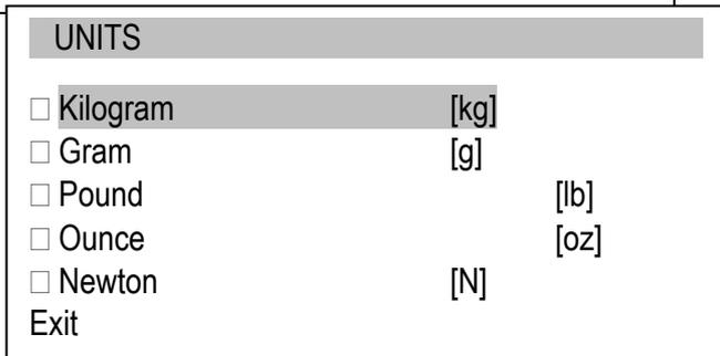
Move the cursor to a mass unit (*kilogram* or *gram*) and press *ENTER*.
