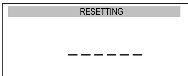
The gauge automatically tests the electronic subassemblies and then resets. During this operation, the gauge should remain stationary and its sensor should not be affected by any forces.
