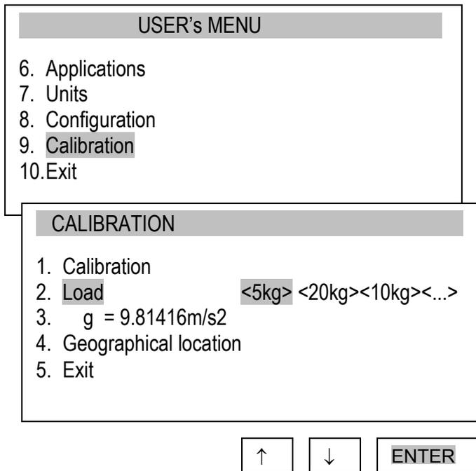
Use the navigation keys and *ENTER* to select *Calibration* and *Load*.
