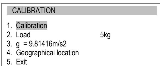
Use the navigation keys and *ENTER* to select *Calibration* and wait until the calibration process is completed.
