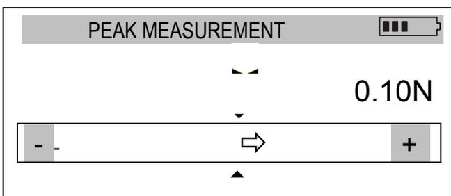
Before starting the measurement, choose a suitable measurement tip, screw it to the gauge plunger and reset the gauge in the operating position, e.g. horizontal position (laying the gauge on a table). The resetting process starts automatically after turning on the gauge or by pressing the  $\rightarrow T(0) \leftarrow$  key.
