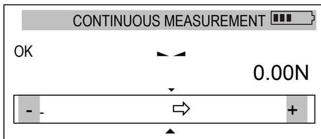
Exit the menu, start the measurement and observe the *MIN*, *OK* and *MAX* indicators on the gauge's display.
