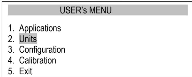
To change force units to mass units, press the *UNIT/CLEAR* or *MENU* key several times. When using the *MENU* key, move the cursor to *Units* and press *ENTER*.
