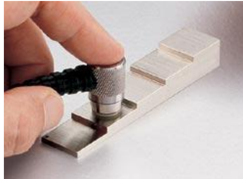
A recalibration of the Material Thickness Meter can be performed with the aid of a calibration block.
