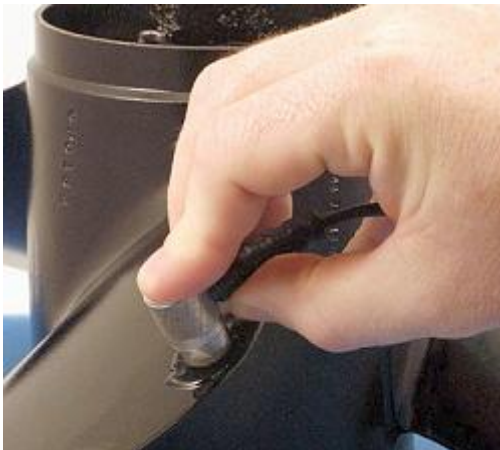
The upper image shows the use of the PT-UTGM Material Thickness Meter in a ship propeller.
